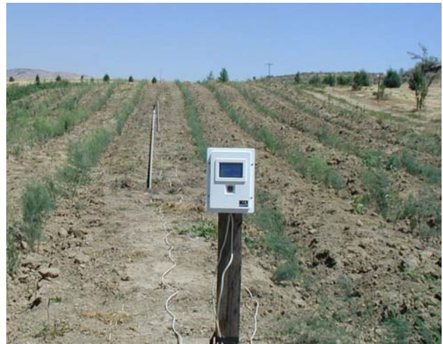
Washington County asparagus field with soil moisture sensors and monitor installed.
