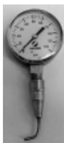
Figure 4. Pitot tube attached to pressure gauge that is used to measure operating pressure of a sprinkler nozzle.
