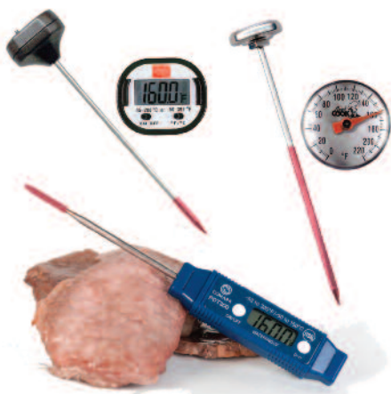
Figure 1. Dial instant-read thermometers (right) sense temperature in the bottom 2 inches of the stem. Digital instant-read thermometers (left and bottom) read temperature in the bottom 1/2-inch of the stem. A thin-tipped thermometer (bottom) can sense the temperature in thin meats.
